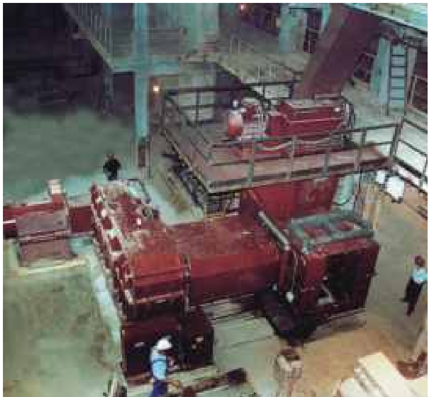
KOMPAKTOR in a factory for potassium chloride. Capacity over 100 to per hour; roll drive motor 800 kW
