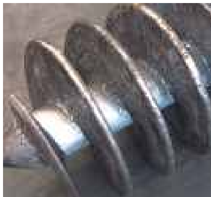
Integral roll Options for alloy overlay against corrosion or welded-on hardfacing.
